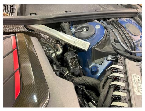
3. You can now rout the supplied harness under the charge pipe at the front driver side of the engine compartment and then under the harness just in front of the performance controller. Then connect the harness to the controller.
