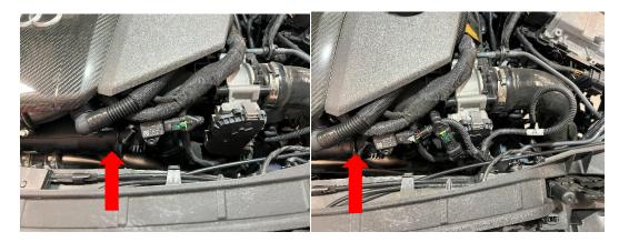
5. Locate the end of the harness that is labeled "B" and rout the harness to the MAP sensor that is on the charge pipe pre throttle body and repeat the previous steps for connecting harness to MAP sensor.
