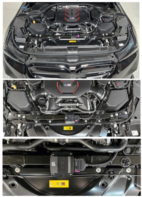
Removing the strut brace bolts provides additional space for connecting the sensors to the harness. Make sure you secure the bolts of the strut brace once the connections are complete.
