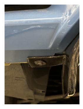
6. After securing the middle section of the diffuser, use the provided double sided tape to help align the side pieces of the diffuser kit to the contour of the car's body lines and the diffuser.
