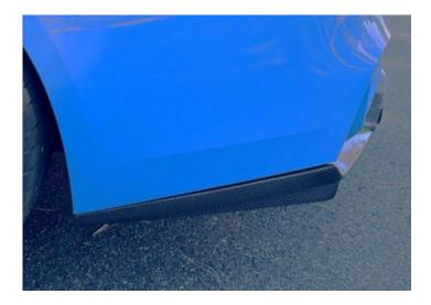
7. After successfully fitting the side pieces of the diffuser kit, use the Phillips head screws provided to securely attach the side pieces of the diffuser kit to the car. Use only the locations where the diffuser has provisions for the hardware. Use double sided tape where it is needed.
