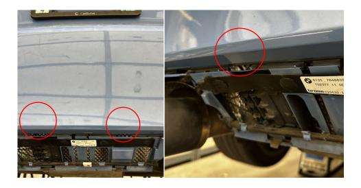
3. Using the holes in the diffuser, located above the exhaust tips, make a note of where to place the provided clips on the heat shield. Remove the rear diffuser to place the clips.
