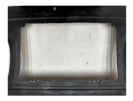
4. When you are done cutting, clean any rough or sharp edges with a file. After finishing the exhaust installation, you can reinstall the undertray, make sure it does not contact the muffler.
