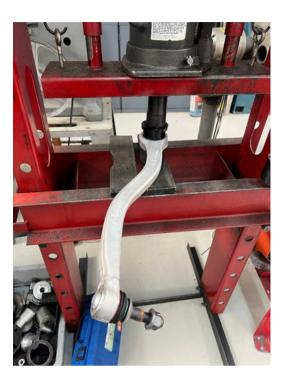
4. Aler pressing the mono ball housings into both arms, you can now locate the threaded hat and M5 hardware provided. Insert the hardware through the mono ball housing and thread into hat locking the housing into the arm. Torque all 8 M5 hardware on both arms to 95-inch pounds in a crisscross paNern. (Note: when torquing hardware in crisscross paNern make sure you go through the sequence at least two Rmes per arm to make sure that the housing and threaded hat have fully seated.)
