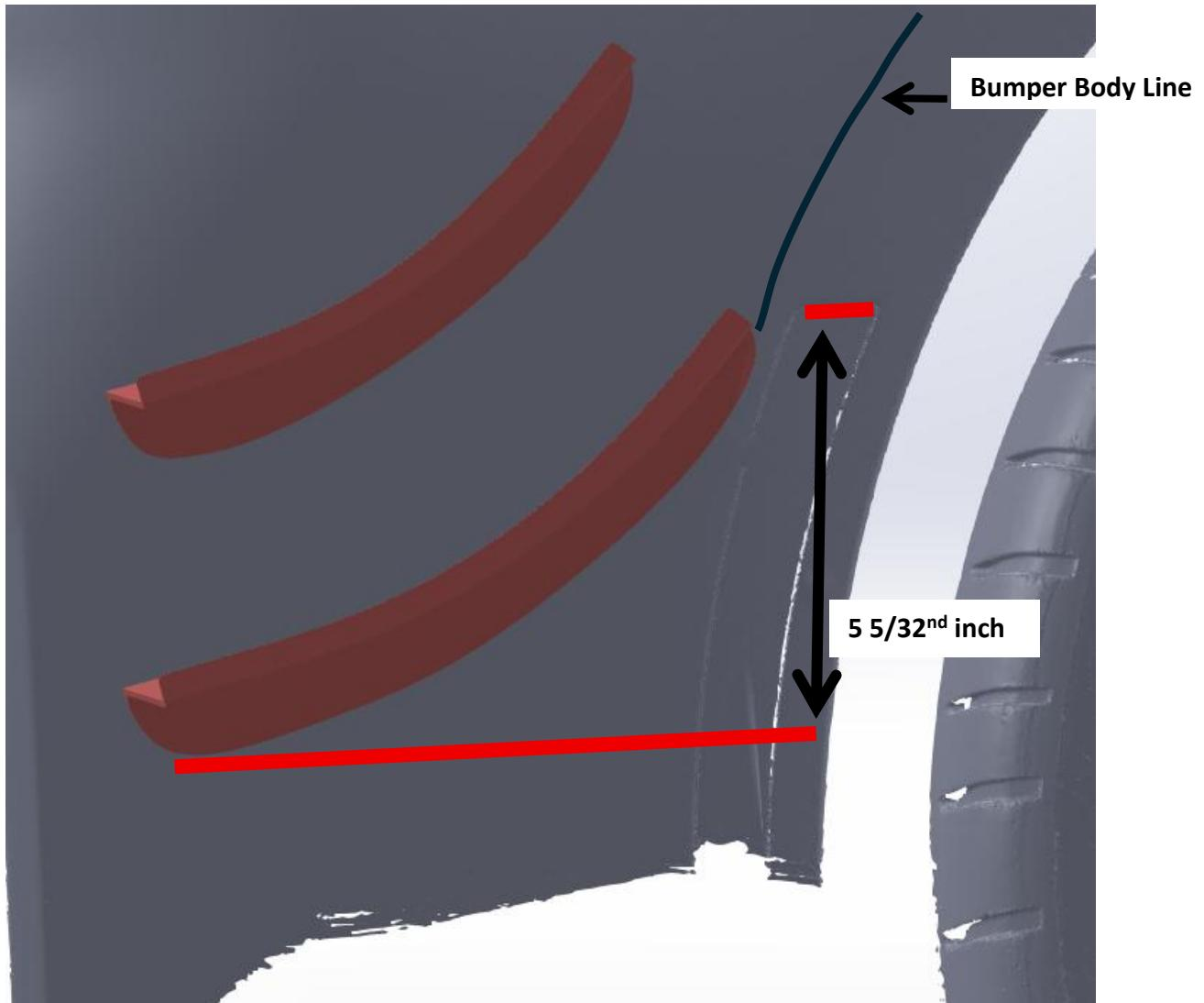
3. The top edge of the lower canard will be in line with the top of the reflector and on the edge of the body line marked above.
