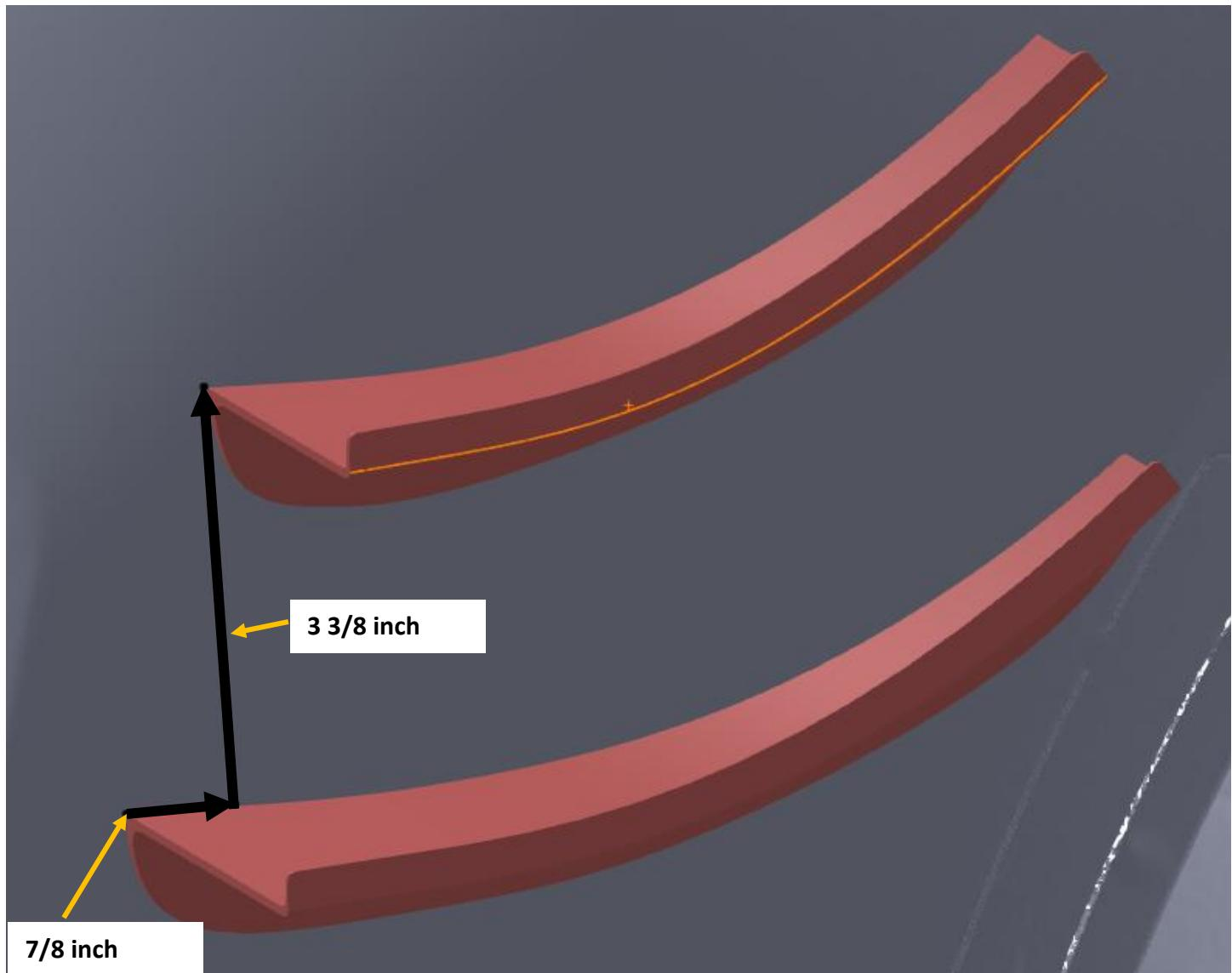
6. Now locate the Left (Driver's side) Upper Canard, you will begin by making your first reference point. From the edge of the lower canard, along the bumper, measure 7/8ths of an inch. From that point go up perpendicularly 3 3/8ths of an inch. This will be where the upper canard edge will be.
