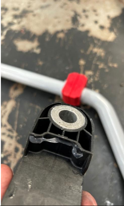
Photo #7 Grease Application (Perform on all edges of both plastic mounts)
