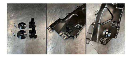
6. After you have completed this process on both sides of the plate you can now reinstall the metal plate back into the car and install the factory hardware and torque to BMW factory spec. (Note: Make sure with the plate fully installed the radiator is moved forward towards the front of the car)
