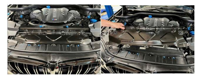
1. The first step in installing the relocation kit is removing the metal plate located at the front of the engine bay that covers the radiator.
