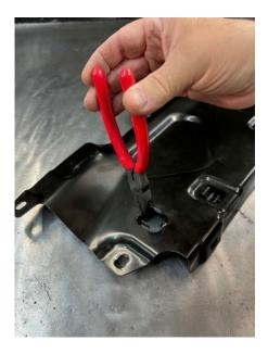
3.Once you have successfully removed the locators, bend the four metal tangs that are on the bottom edge of the hole where the plastic locators were previously installed so that they are vertical. You can accomplish this by grabbing the tangs with a pair of plyers and bending the tang away from the whole. (NOTE: The tangs only need to be bent away from the hole a minimal amount.)
