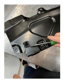
2. With this plate out of the car and sitting face down on a bench you can remove the two plastic radiator locators on both ends of the plate by depressing the plastic tabs using a couple of flat blade screwdrivers.
