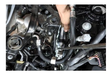
Note: The A/C lines that run between the engine and the strut tower may make getting the right angle to remove the MAP sensor screws difficult, you can slightly flex the lines out of your way to make the screws more accessible. Make sure to not apply too much pressure that would cause any form of damage to the A/C lines.
