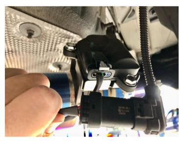
Squeeze the release tab on the stock plug and remove it from the exhaust valve, plug this stock plug into the female end of the controller harness. Then plug the male end of the controller harness into the exhaust vale
