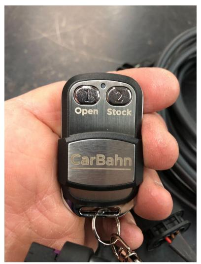
The Kit comes with two identical key fob remotes for the valve controller. Slide the cover down on the remote to expose the buttons.
