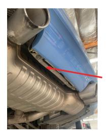
If you are doing a two valve kit note that the wiring harness has a long and short leg, rout the short leg to the valve closest to the box and the long leg of the harness to the valve on the other side. The far side harness can be run under the heat shield that is above the muffler, by removing the screws that attach the shield to the bumper and the small nuts that attach the shield to the car above the muffler.
